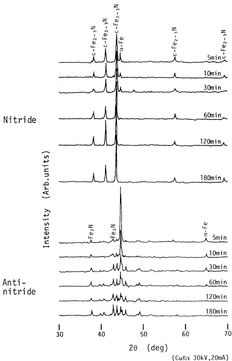
Figure 3 Diffraction intensity curves obtained by X-ray.
