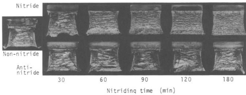
Figure 6 Macroscopic impact fracture surfaces (20°C).
