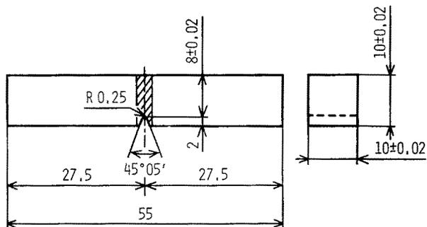
Figure 1 Test specimen (size in mm).
