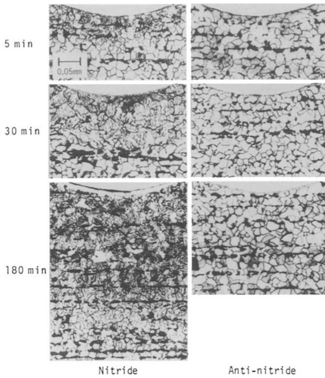
Figure 4 Microstructures in the vicinity of notch roots (tempered at 300°C for 60 min).
