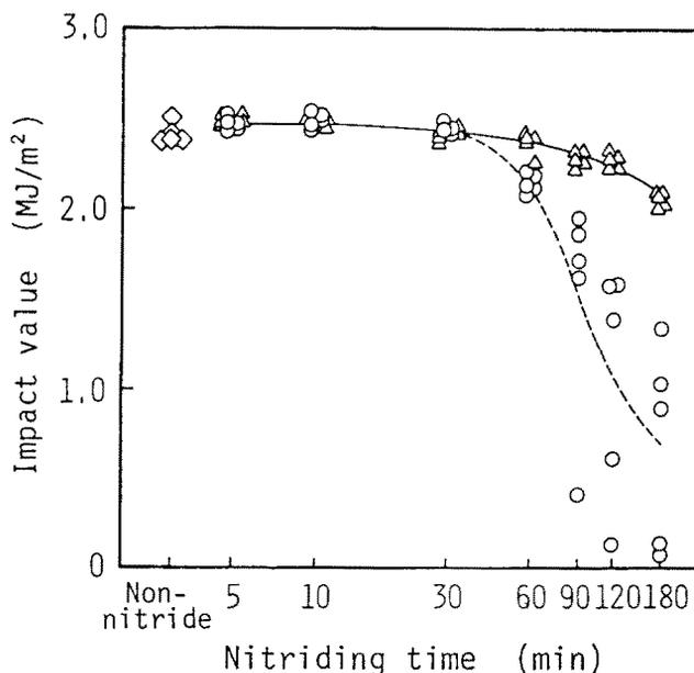
Figure 5 Relation between Charpy impact value and nitriding time (20°C). (---○---) nitride; (---△---) anti-nitride.
