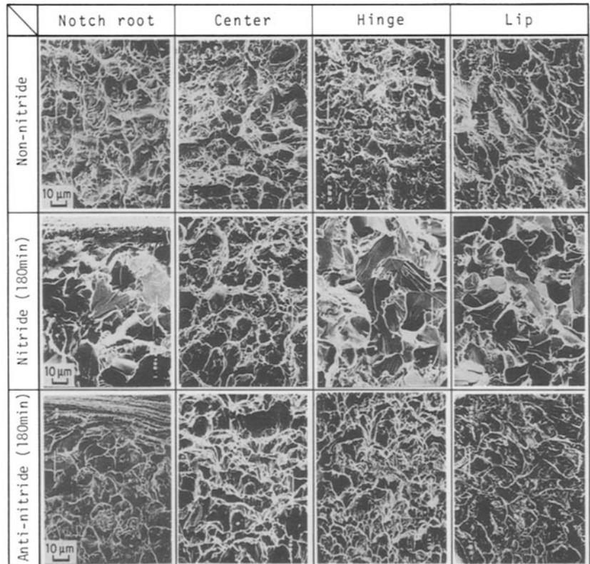
Figure 7 SEM photomicrographs of fracture surfaces.
